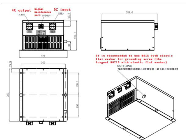
3.2 Inverter module port definition and power distribution installation
